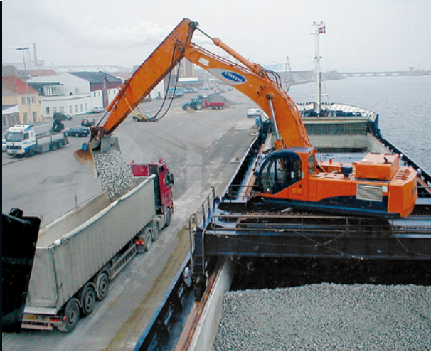
DISCHARGING SPLIT TO LORRIES
